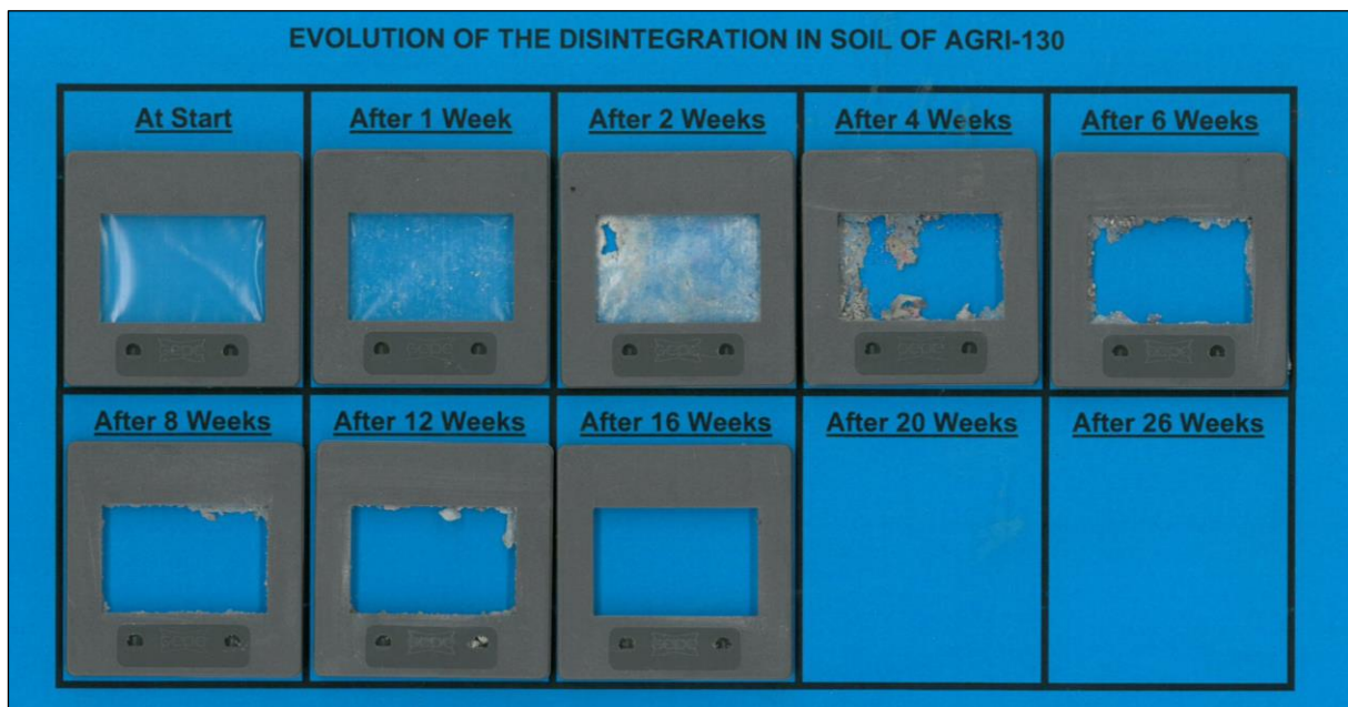
Figure 60: Visual presentation of the evolution of the disintegration of test material Trilayer film A/B/C; A and B = PBSA +10%PBAT, C= PBSA+5%oligomer + 10% PBAT (45 \mu\text{m} ), put into slide frames, during the incubation process in soil
