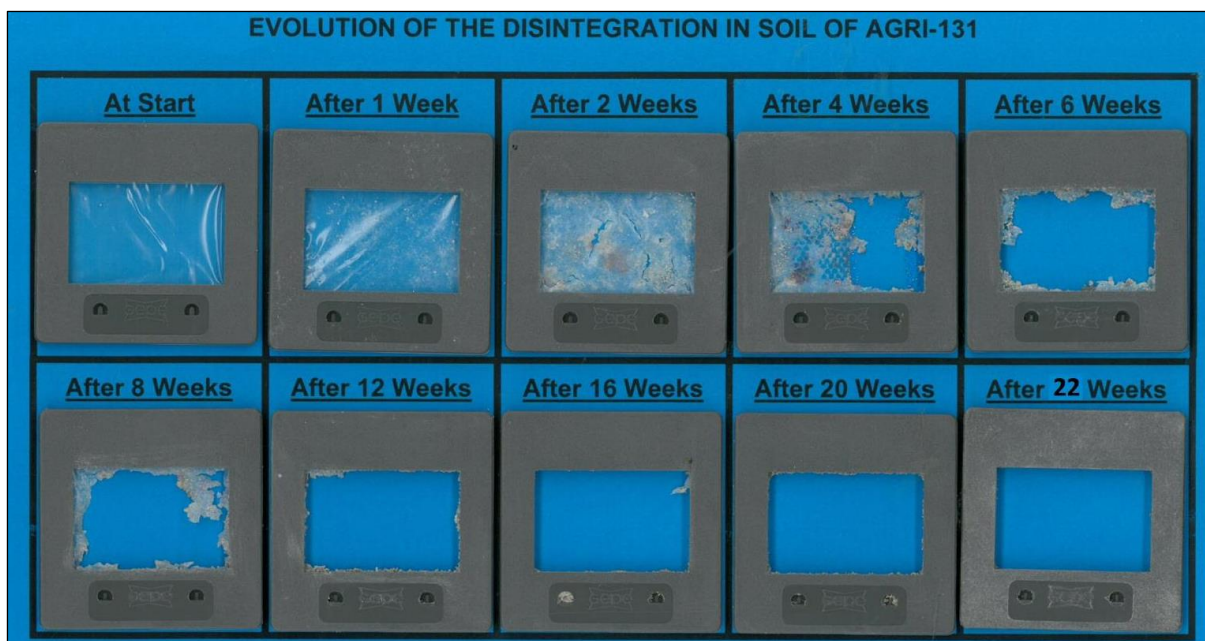
Figure 61: Visual presentation of the evolution of the disintegration of test material Trilayer film A/B/C; A and B = PBSA +10%PBAT; C= PBSA+5%oligomer (45 \mu\text{m} ), put into slide frames, during the incubation process in soil.
