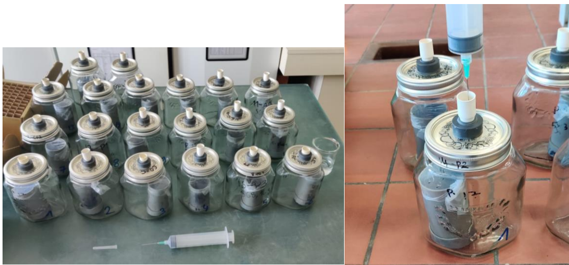
Figure 14. On the left the closed sample jars with incubation cylinders inside. On the right a sample jar with sample syringe.
