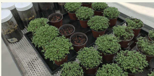
Fig. 1: Closed and open cress test, 7 days after sowing, ready for evaluation.
