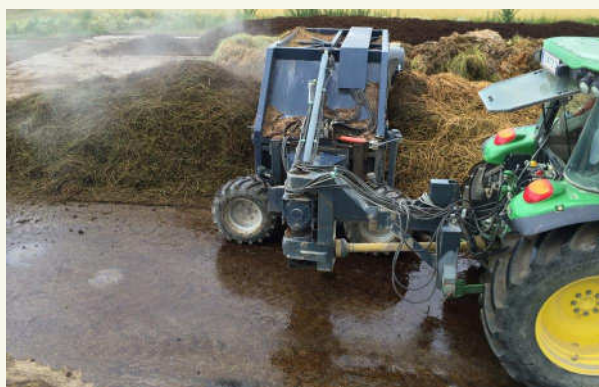
Fig. 1: Homogenizing resources for thermophilic compost production with a compost turner
