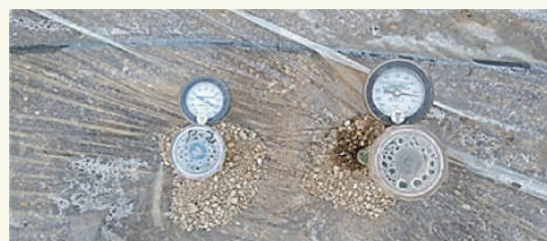
Fig. 1: Tensiometers to measure the soil humidity during solarisation. The left one is placed at 15 cm-depth, and the right one at 35 cm-depth.
